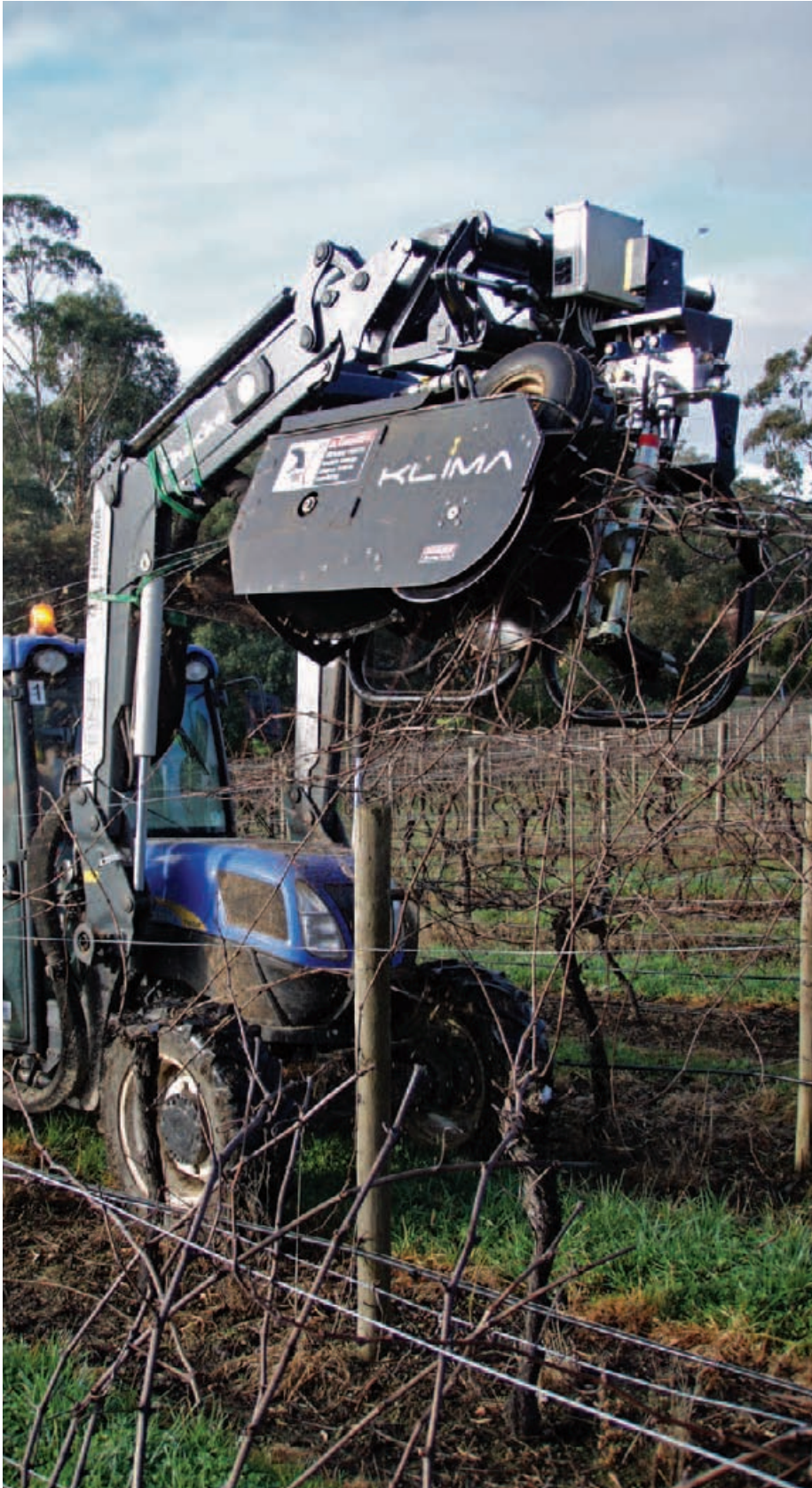
The Klima machine, which went on sale this year, is one of two machines developed recently to physically strip the previous season's canes out of the vertically shoot positioned (VSP) foliage wires.
